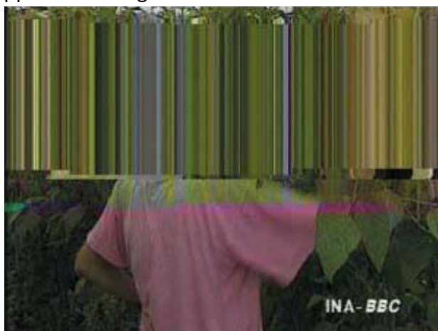
Figure 14: Exemple de drop-out dans un enregistrement en Betacam analogique (Kokaram, On Missing Data Treatment for Degraded Video and Film Archives: A Survey and a New Bayesian Approach 2004)
